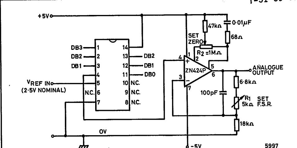
Fig. 3 6-bit D-A converter
