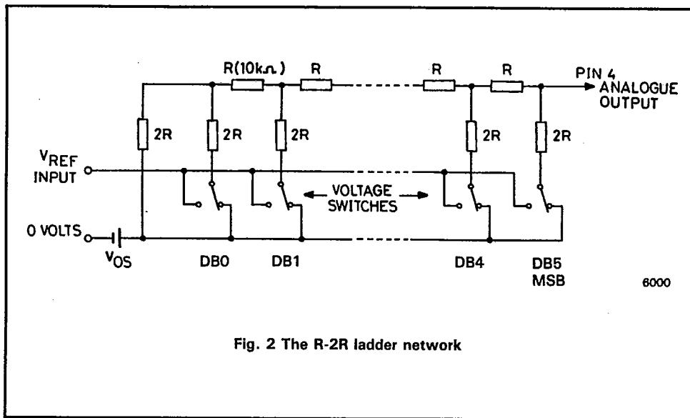
Each 2R element is connected either to OV or  $V_{REF}$  by transistor switches specially designed for low offset voltage (typically 1mV).
