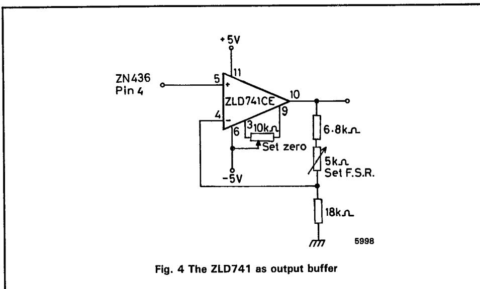
Fig. 4 The ZLD741 as output buffer
